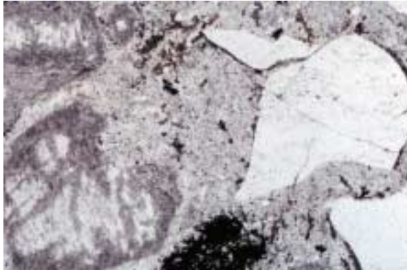
Figure 4a. Fragmental rhyolite (OS17). Broken alkali feldspar and quartz phenocrysts in a fine-grained fragmental groundmass composed of quartz and feldspar. Minor biotite. Plane light. Width of field of view, 5 mm.
