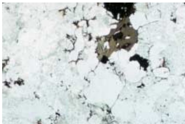
Figure 7a. Medium- to coarse-grained, phaneritic, pink granite (OS44). Quartz, alkali feldspar, and brown biotite. Plane light. Width of field of view, 5 mm.
