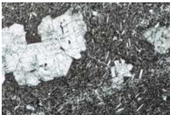
Figure 3a. Porphyritic basalt (OS14). Plagioclase and pyroxene phenocrysts in a flow-banded plagioclase and pyroxene groundmass. Plane light. Width of field of view, 5 mm.
