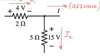
Conserv. of current at the junction point:  $\Sigma_i T_{in} = \Sigma_i T_{out}$  $T_i = I + I_2 = 2A = I + 3A = I = -1A$
