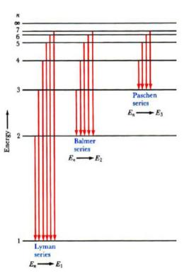
In this lab we will analyze the visible spectrum that are emitted by the hydrogen atom (Balmer series).
