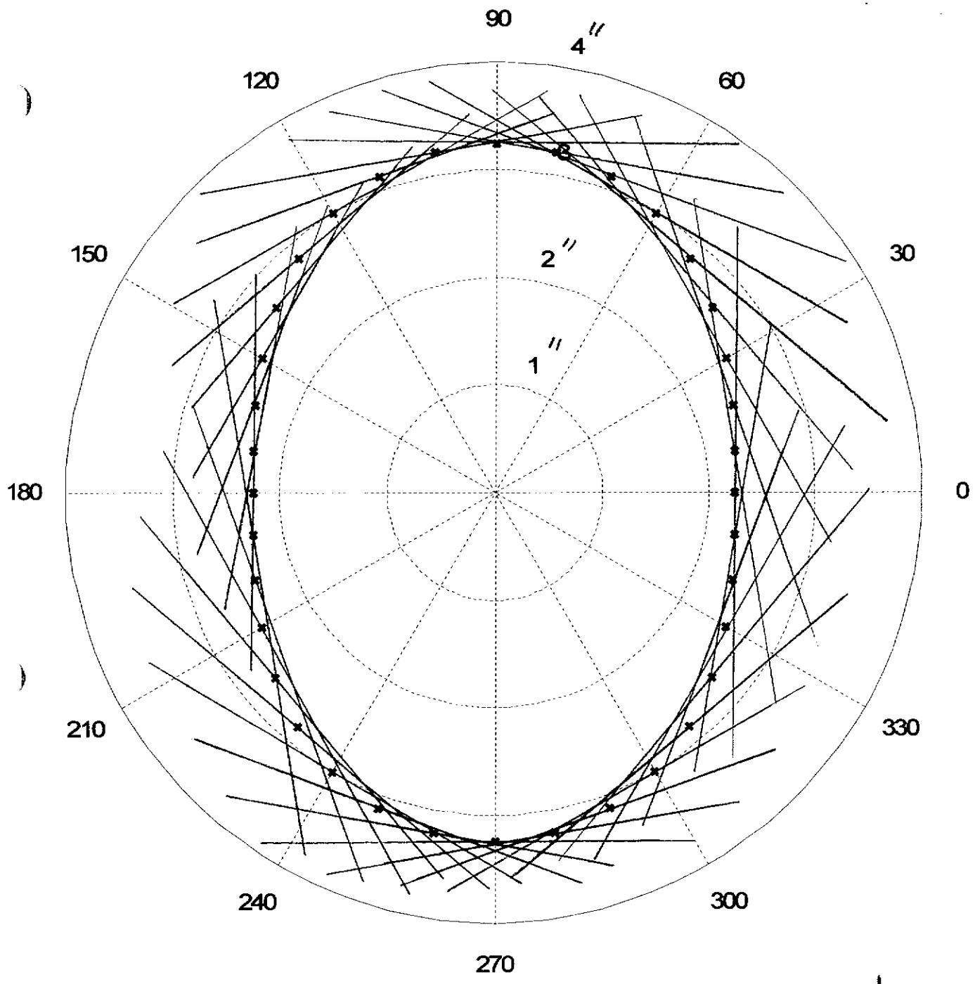
The cam shape is inscribed within the tangent lines. It should be smooth and touch all the lines, otherwise the cam is undercut.
