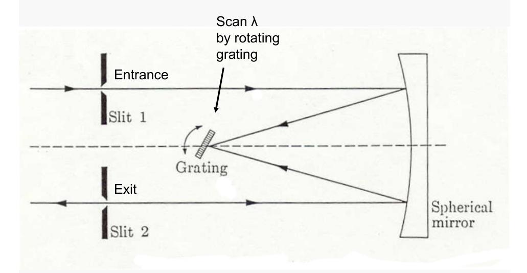
Littrow mounting is the same as for prism except use grating in place of prism Grating Characteristics – Resolution & Dispersion are very high for a long, finely ruled grating
