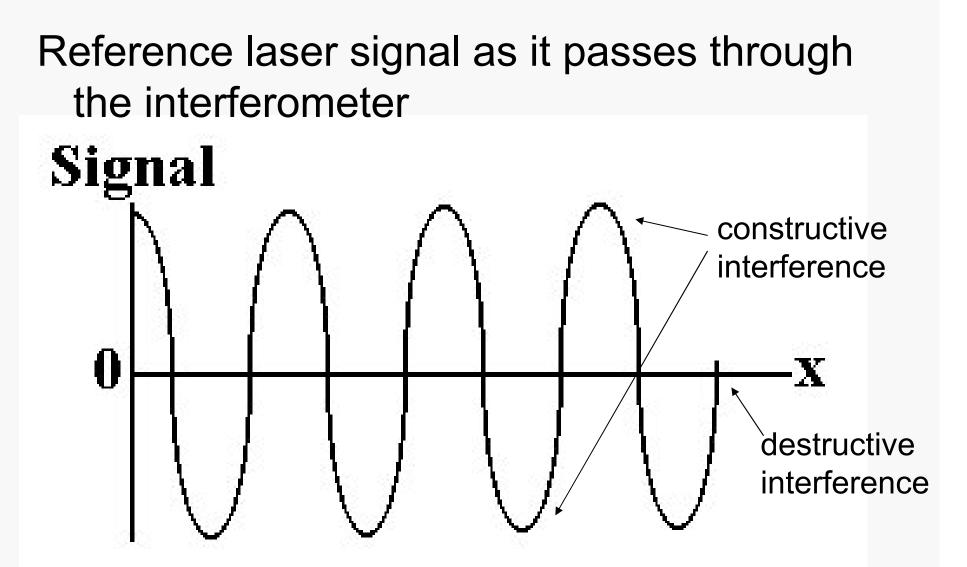
This allows the position of the moving mirror to be determined accurately
