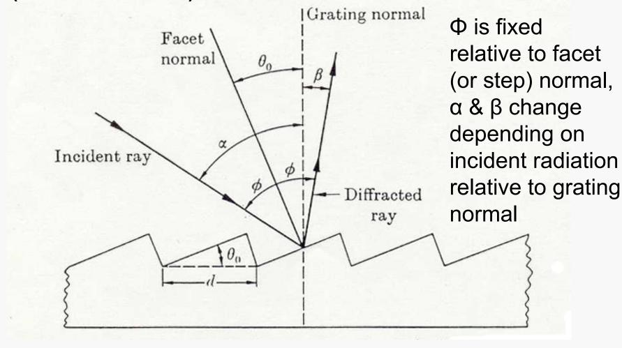
Preparation of reflection gratings – a master grating is prepared by ruling grooves in a reflective aluminum surface on glass (from 20 – 3000 grooves/mm or 10,000 lines/inch)
