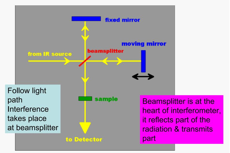
Interferometers have no slits so a wide beam of radiation can be used
