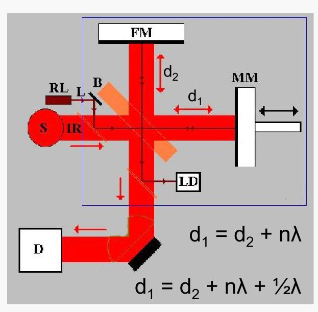
Where: S = IR sourceIR = infrared beam D = detectorB = beamsplitter FM = fixed mirror MM = moving mirror RL = reference laser L = laser beamLD = laser detector  $d_1$  = distance to moving mirror  $d_2$  = distance to fixed mirror
