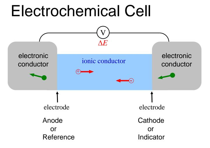
(V) - Represents device to measure potential (voltage) without drawing significant current i.e potentiometer or electrometer (high input impedance  $\geq$  100 M $\Omega$ (mega ohms)
