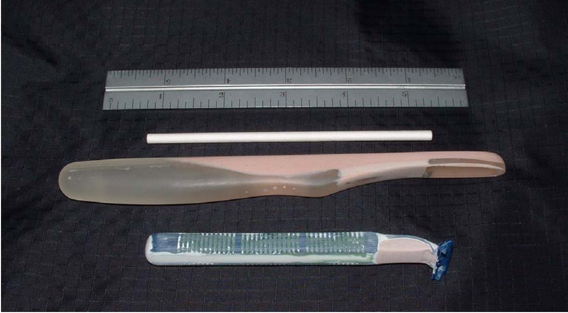
Figure 5: Modified models for toothbrush and razor handles shown with cardboard rod stiffener.
