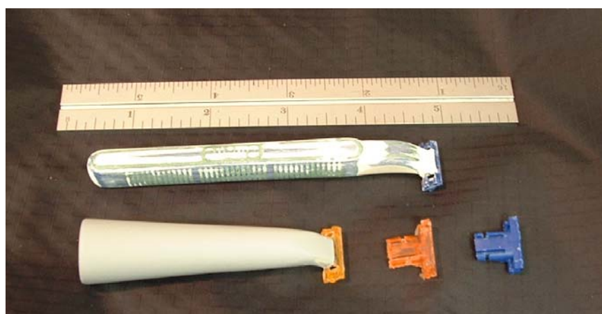
Figure 4: Two designs for razor handles shown with the hard plastic inserts used to attach the blade holder.
