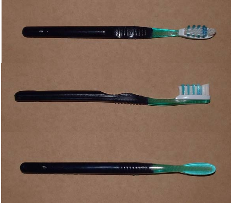
Figure 1. Thermosetting polymer toothbrush prototype with soft handle.
