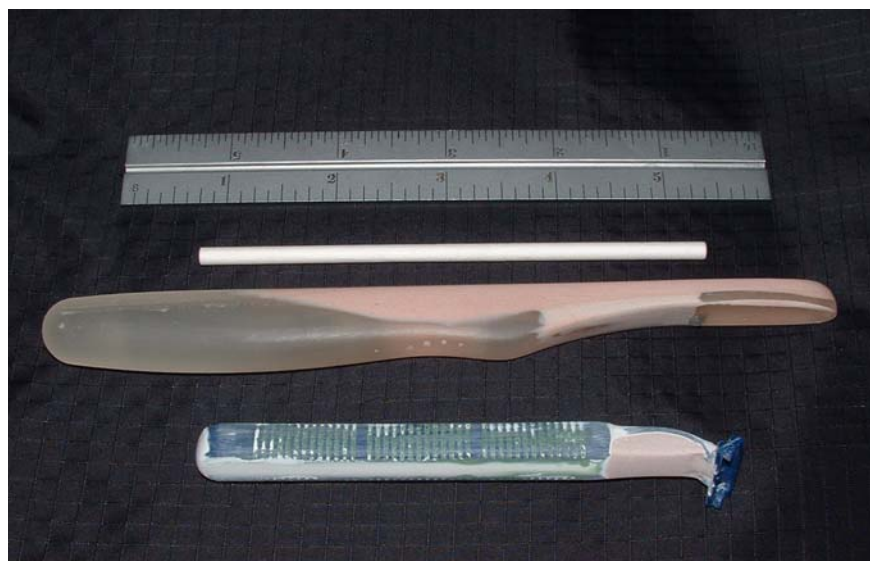
Figure 3: Modified models for toothbrush and razor handles shown with cardboard rod stiffener.
