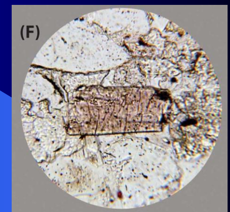
Tourmaline absorbs more light when the long axis of the crystal is perpendicular to the polarizer.
