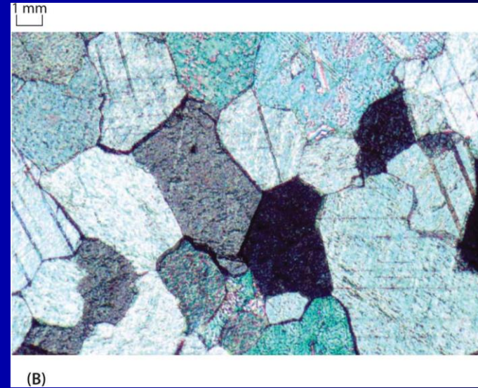
Marble showing 120° grain boundary junctures
