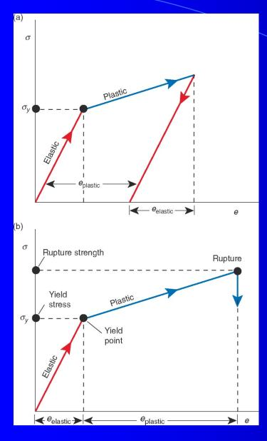
Plastic strain is the permanent change in shape or size of a body without fracture, accumulated over time by a sustained stress beyond the elastic limit (yield point) of the material.
