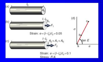
Hooke's Law:  $\sigma = \text{Ee}$   $\sigma = \text{stress}$  E = Young's moduluse = extension (one-dimensional strain)
