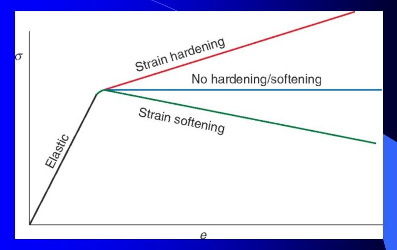
The blue curve represents creep which occurs when the material continues to deform without any increase in the applied force or stress.
