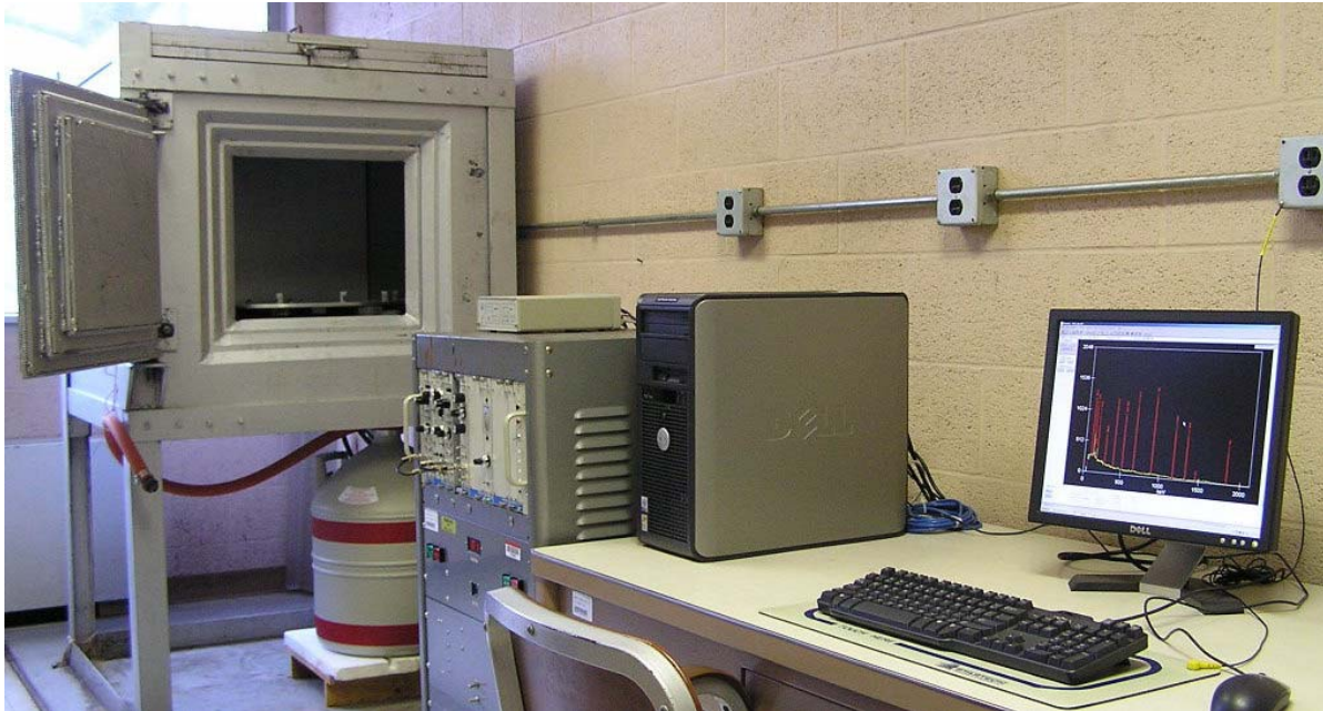
Figure 4. Gamma-ray spectroscopy system (automated sample changer). The detector is kept at liquid nitrogen temperatures (dewar under cave). The small box on top of the cabinet combines all the functions of the HV power supply, spectroscopy amplifier, and analog-to-digital converter. The resultant spectrum is shown on the computer screen.
