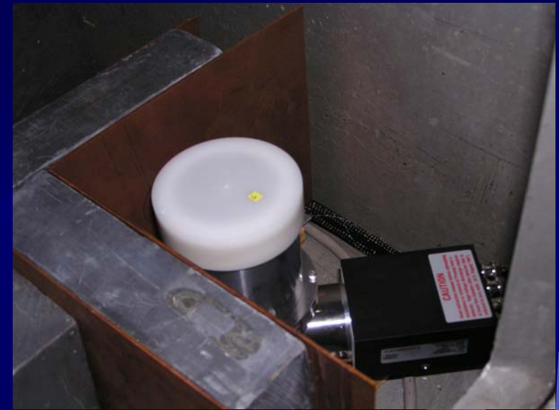
Detector positioned in shielded well
