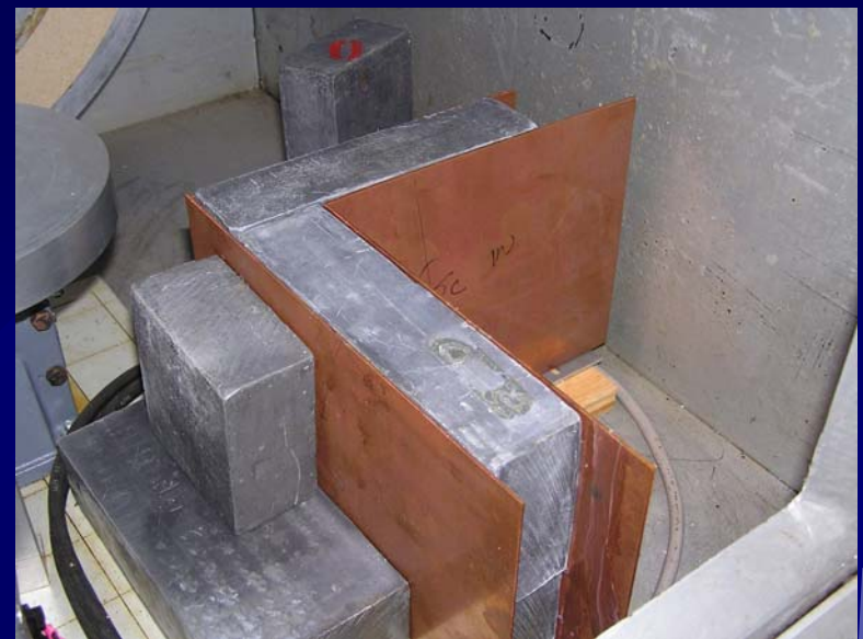
Pb and Cu shielding in detector well
