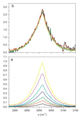
Fig. 3. Measured absorption coefficients (bottom) and associated square density normalized values (top) for pure  $CO_2$  at 295.15 K and seven total pressures from 15 to 44 atm: (b) Dens normalized Abs  $(10^{-6} \text{ cm}^{-1}/\text{atm}^2)$  and (a) Abs Coeff  $(10^{-2} \text{ cm}^{-1})$ .
