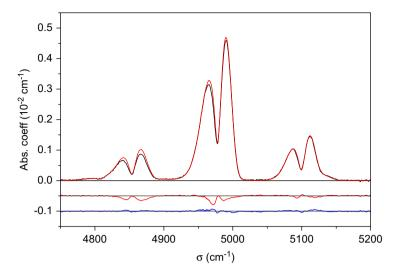
Fig. 4. Measured (—) and calculated (——, with the former version of our database and software) absorption coefficients for 1%  $CO_2$  in 18.3 atm of  $N_2$  at 295.15 K in the region of the  $2\nu_1+\nu_3$  triad. The lower traces give the shifted meas-calc residuals obtained with the former (——) and new (——) version of our database and software.
