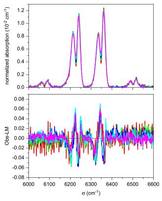
**Fig. 7.** Absorption coefficients and meas-calc residuals for 10% CO<sub>2</sub> in five pressures (from 30 to 76.0 atm) of N<sub>2</sub> at 295.15 K in the region of the  $(3\nu_1+\nu_3)$  tetrad. The top panel displays the measured absorptions normalized to unity area through integration over  $\sigma$ . The lower panel displays the residuals (meas-calc) obtained from calculations with our new database taking line-mixing into account.
