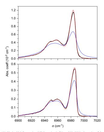
**Fig. 8.** Absorption coefficients for 10% CO<sub>2</sub> in: 29.9 (bottom) and 72.3 atm (top) of N<sub>2</sub> at 295.15 K in the region of the  $3v_3$  band. — are measured values, whereas — and — have been calculated with the new version of our database and software, respectively, neglecting line-mixing and taking this process into account.
