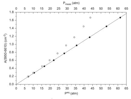
**Fig. 2.** Integrated intensity (area) between 5950 and 6610 cm<sup>-1</sup>, obtained from pure  $CO_2$  measurements (Fig. 1) at 295.2 K, plotted vs the measured pressure  $P_{\text{meas}}$  ( $\bigcirc$ , top x-axis) and the equivalent pressure  $P^{\text{eq}}$  ( $\bigcirc$ , bottom x-axis). The line corresponds to the law  $S(5950,6610) = 0.02722 \times P^{\text{eq}}$ .
