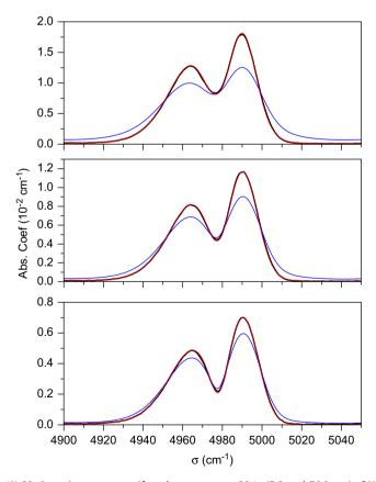
**Fig. 5.** Absorption coefficients for 1%  $CO_2$  in various pressures (from bottom to top: 28.1, 47.6, and 76.0 atm) of  $N_2$  at 295.15 K in the region of the  $(2\nu_1 + \nu_3)_2$  band. — are measured values, whereas — and — have been calculated with the old and new version of our database and software, respectively, neglecting line-mixing and taking this process into account.
