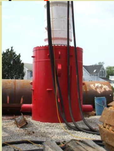
IHC S-600 Hydraulic Hammer: Rated Energy ~440kip-ft (600kN-m)
