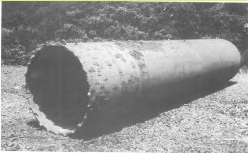
Figure 4.11 A typical single-walled core barrel (O'Neill & Reese, 1999)
