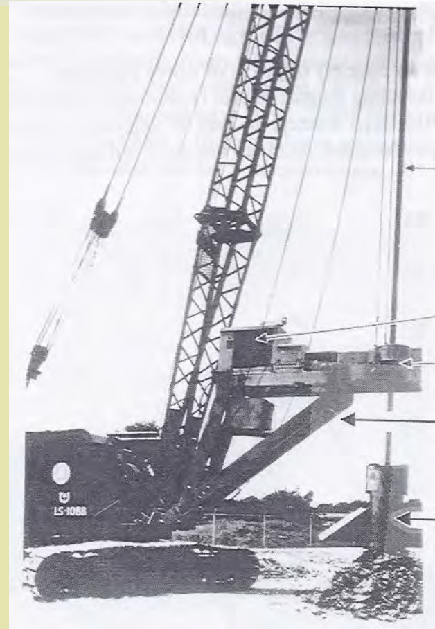
Figure 4.2 A typical crane-mounted drilling machine (Photograph courtesy of Farmer Foundation Company, Inc.) (O'Neill & Reese, 1999)
