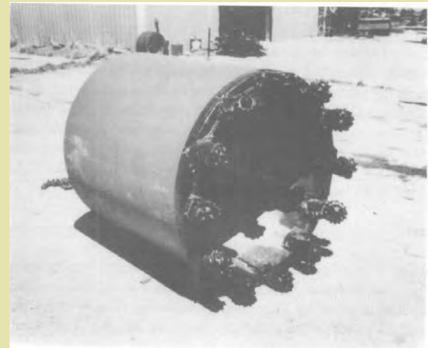
Figure 4.12 A double-wall core barrel (Photography courtesy of W.F.J. Drilling Tools, Inc.) (O'Neill & Reese, 1999)
