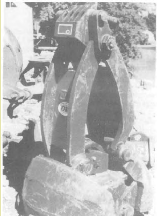
Figure 4.17 A typical grab bucket (Photography courtesy of John Turner) (O'Neill & Reese, 1999)
