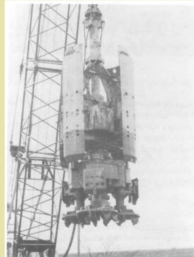
Figure 4.20 An example of a rodless soil drill (Photography courtesy of Tone Boring Corp., Ltd.) (O'Neill & Reese, 1999)
