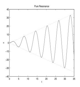
3. (Resonance) Consider a mass-spring system with mass m = 1 kg, spring constant k = 1 N/m, damping constant c = 0.1 N·sec/m, and external force  $F(t) = \cos(\omega t)$  N, where
