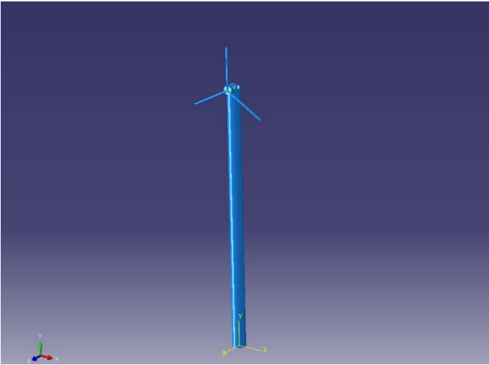
Fig. 5: Finite element model of the wind turbine (rendered beam profile image from Abaqus/CAE™)
