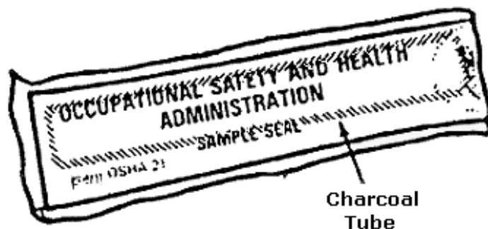
FIGURE II:1-4a. CORRECTLY SEALED C-TUBE. SAMPLE IS COMPLETELY ENCLOSED IN THE SEAL, AND NO TAMPERING IS POSSIBLE.
