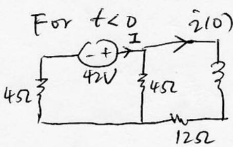
$$R_{\text{eq}} \text{ w.r.t } \text{ ground} = 4 + 4/12 = 7\Omega$$
