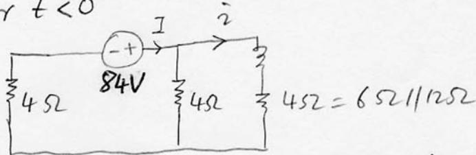
$$R_{eq} \text{ w.r.t } t \quad R_{eq} = 4 + 4/14 = 6.52$$
