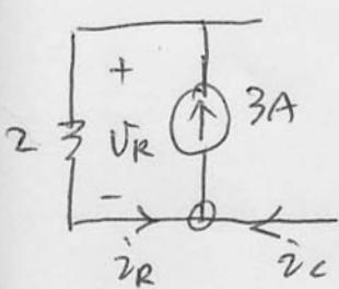
$$\begin{aligned} V_R(t) &= 2(3 - 0.25 \times (16e^{-t} - 8e^{-2t})) \\ &= 6 - 8e^{-t} + 4e^{-2t} \text{ V} \end{aligned}$$
