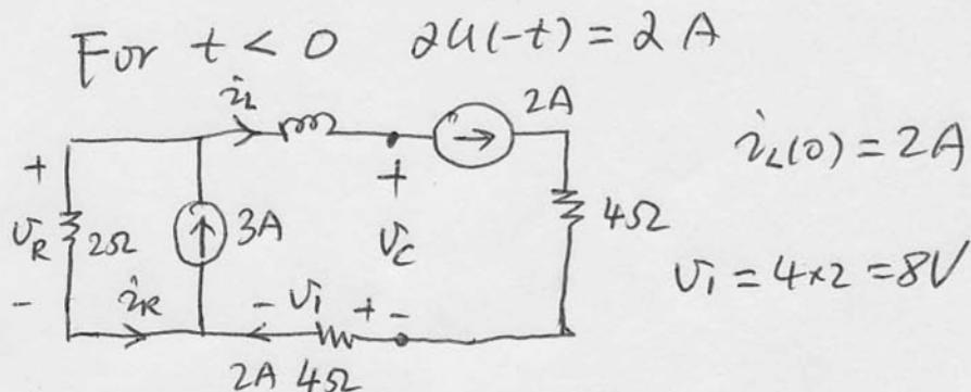
$$\text{By KCL, } i_R = 3 - 2 = 1 \text{ A}, \quad V_R = 2 \text{ V}$$
