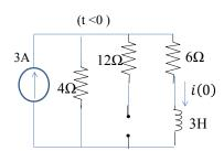
For t < 0, under DC condition, inductor is short circuit.
