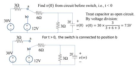
Find  $v(\infty)$  as the capacitor voltage under DC condition. Also by voltage division:
