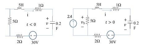
For t < 0, 2u(t)=0A, current source off (open circuit)
