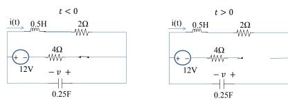
It is more convenient to find capacitor voltage first. Then take derivative to find loop current. Assign capacitor voltage as in figures.
