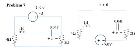
Step 1: For t < 0, 4u(-t) = 4A, current source on; 60u(t) = 0V, voltage source off (short).  $v(0) = -4 \times 6V = -24V$ , i(0) = 0, v'(0) = 0.
