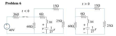
Step 1: Find v(0) and inductor current i(0) from circuit for t<0. Since no voltage across  $6\Omega$ , v(0) is the same as voltage across  $60\Omega$ , which is in parallel with  $15\Omega+25\Omega$ ,  $60//(15+25)\Omega=24\Omega$  By voltage division,
