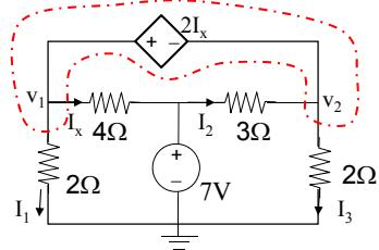
$$I_1 = \frac{v_1}{2}; \quad I_2 = \frac{7 - v_2}{3};$$
