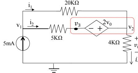
There is an additional voltage  $v_3$  which is different from  $v_1, v_2$ . Due to the floating voltage source, form a super-node.
