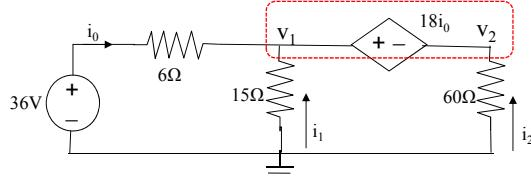
Due to the floating dependent voltage source, a super-node need to be formed
