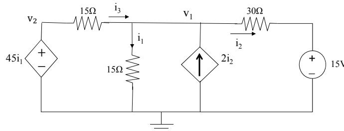
$$\text{Assign } v_2, \text{ Then } v_2 = 45i_1 \quad (1)$$
