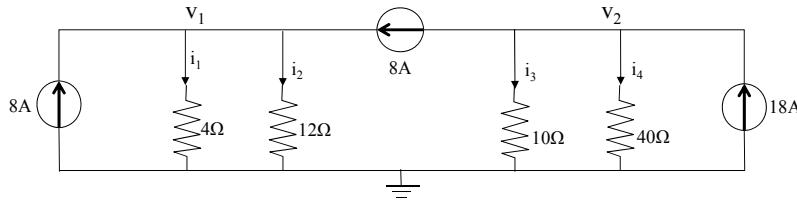
KCL at  $v_1, v_2$ :  $i_1 + i_2 = 8 + 8 = 16$ ;
