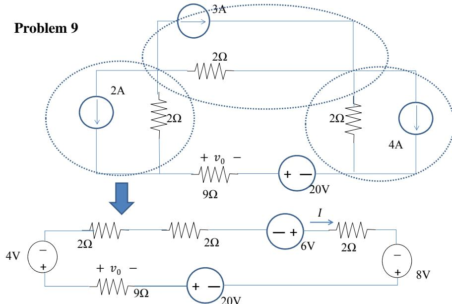
$$\text{Loop current: } I = \frac{20+8+6-4}{2+2+2+9} = \frac{30}{15} = 2A; \quad v_0 = -9I = -9 \times 2 = -18V$$
