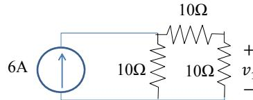
$$v_2 = 3 \times \frac{10}{10+20} \times 10 V = 10V$$
