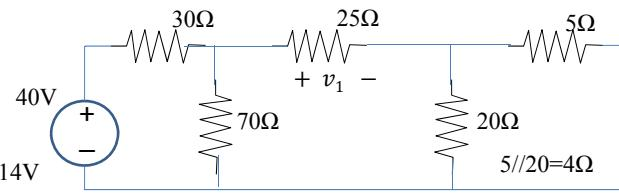
$$v_2 = -\frac{46||20}{46||20+5} \times 20 \times \frac{25}{25+21} V = -8V$$
