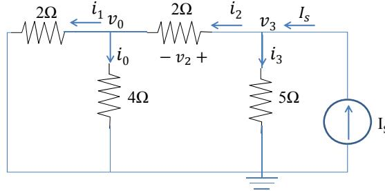
Pick the ground and assign node voltages, resistor voltages and currents
