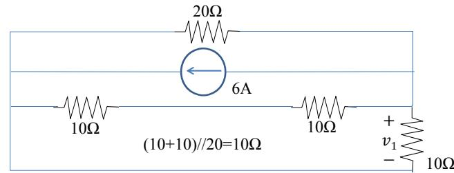
$$v_1 = -6 \times \frac{10}{10+10} \times 10 = -30V$$
