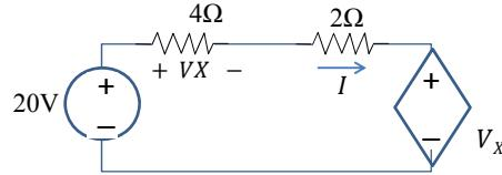
$$V_x = 4I; \\ \text{KVL: } V_x + 2I + V_x = 20; \\ 4I + 2I + 4I = 20; \\ I = 2A; \\ V_x = 4I = 8V$$
