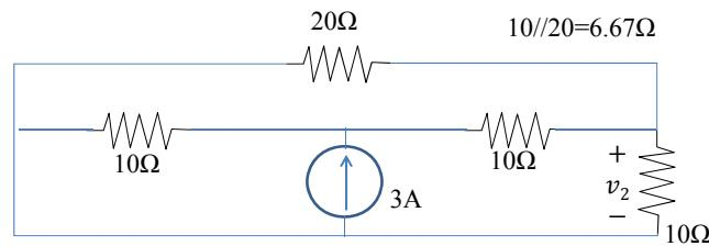
$$v_2 = 3 \times \frac{10}{6.67+10+10} \times \frac{20}{10+20} \times 10 = 7.5V$$
