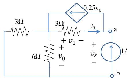
$$V_{TH} = 3V, R_{TH} = 3.5\Omega$$
