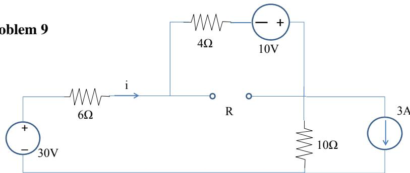
Need to compute Thevenin's equivalent with respect to the two terminals:
