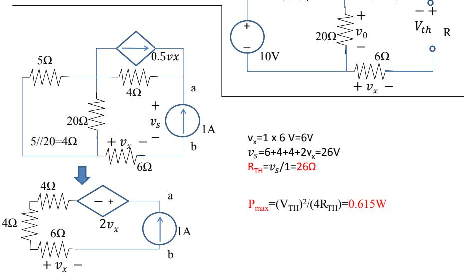
$$v_x = 1 \times 6 \text{ V} = 6 \text{ V}$$
