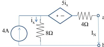
To find  $R_N$ , turn off 4A, supply 1A source, need to find  $v_0$
