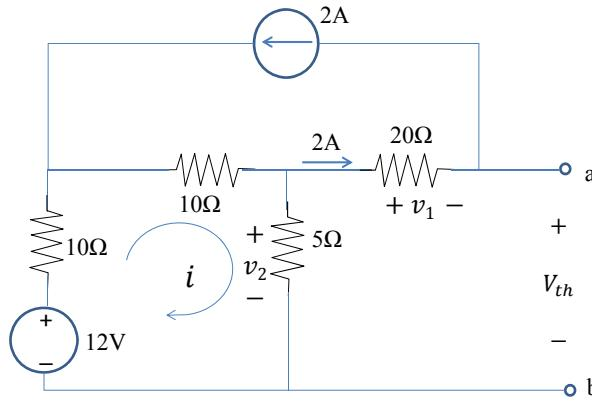
$$-12 + 10i + 10(2+i) + 5i = 0 \\ \Rightarrow i = -0.32A \\ v_2 = 5i = -0.32 \times 5 = -1.6V \\ V_{TH} = v_2 - v_1 = -1.6 - 40 = -41.6V \\ R_{TH} = 20 + 5/(10+10) \Omega = 24\Omega$$
