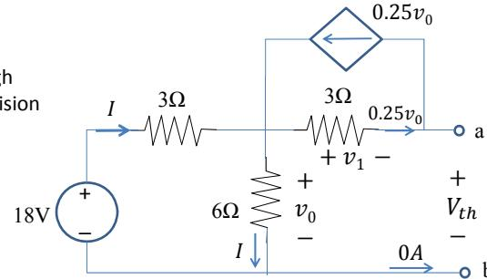
To find  $R_{th}$ , turn off 18V, supply 1A source, need to find  $v_s$ . In this case  $3\Omega$  and  $6\Omega$  are in parallel
