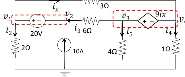
Due to the two floating voltage sources, two supernodes need to be formed:
