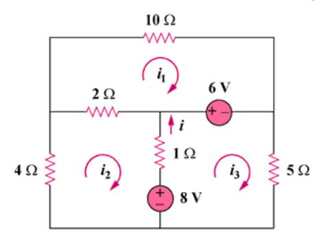
KVL along mesh 1:  $10i_1 - 6 + 2(i_1 - i_2) = 0$  (note:  $i_1$  terms with "+")  $\rightarrow 12i_1 - 2i_2 = 6$  (1) Mesh 2:  $2(i_2 - i_1) + 1(i_2 - i_3) + 8 + 4i_2 = 0$  ( $i_2$  terms with "+")  $\rightarrow -2i_1 + 7i_2 - i_3 = -8$  (2) Mesh 3:  $6 + 5i_3 - 8 + 1(i_3 - i_2) = 0$  ( $i_3$  terms with "+")  $\rightarrow -i_2 + 6i_3 = 2$  (3)
