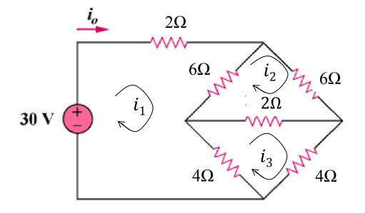
Use the short cut without assigning resistor voltages: KVL along mesh 1:  $2i_1 + 6(i_1 - i_2) + 4(i_1 - i_3) - 30 = 0$  (note:  $i_1$  terms with "+") Simplify to get  $\rightarrow 12i_1 - 6i_2 - 4i_3 = 30$  (1)
