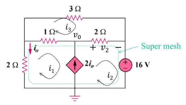
First, express controlling current  $i_0$ :  $i_0 = -i_1$  (0) KVL along mesh 3:  $3i_0 + 2(i_0 - i_0) + (i_0 - i_1) =$
