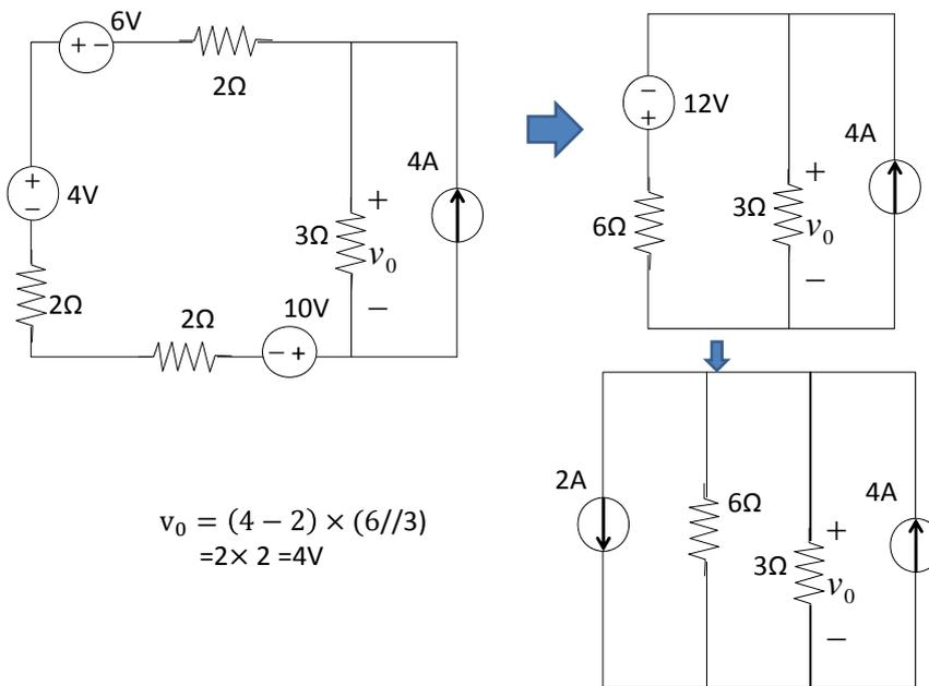
$$v_0 = (4 - 2) \times (6/3) = 2 \times 2 = 4V$$
