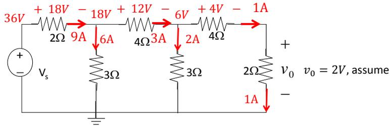
Step 1: Find  $k$  such that  $v_0=kV_s$  by assuming  $v_0=$  some value
