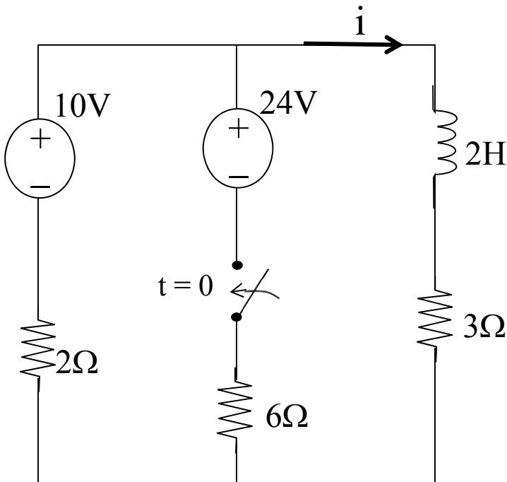
$$A: \begin{aligned} i(0) &= 2A, i(\infty) = 3A, R_N = 4.5\Omega \\ i(t) &= 3 - e^{-2.25t} A \end{aligned}$$
