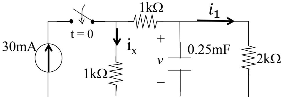
$$A: \begin{aligned} v(t) &= 15(1 - e^{-4t})V \\ i_x(t) &= 22.5 \times 10^{-3} - 7.5 \times 10^{-3}e^{-4t}A \end{aligned}$$
