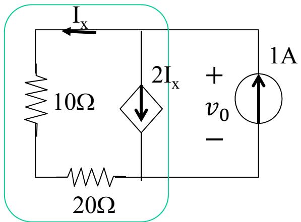
$$I_x + 2I_x = 1, \rightarrow I_x = \frac{1}{3} A, v_0 = 10V$$
