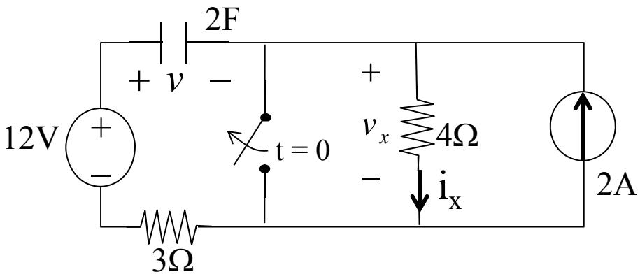
$$A: \begin{aligned} v(t) &= 4 + 8e^{-t/14}V \\ i_x(t) &= 2 - (8/7)e^{-t/14}A \end{aligned}$$
