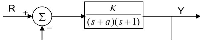
Find  $a$  and  $K$  so that the overshoot is less than 10% and the settling time is less than 1 second. You may use the  $M_p - \zeta$  graph for your design.
