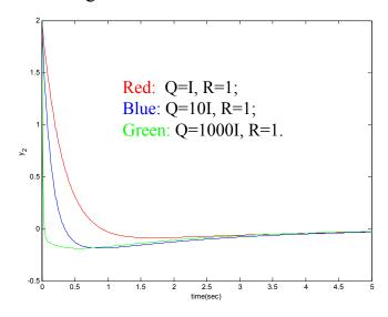
Simulation with feedback from estimated state Control u: larger Q results in larger magnitude of u
