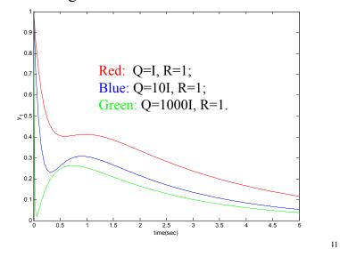
Output  $y_2$ : Larger Q results in faster convergence rate of y and smaller magnitude
