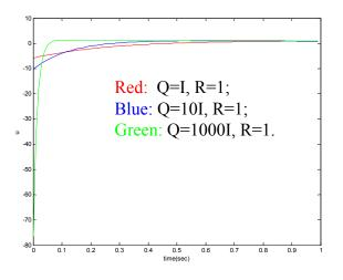
Output  $y_1$ : Larger Q results in faster convergence rate of y and smaller magnitude
