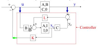
The inputs to the controller are u and y, the output is  $Kx_{e}$  25
