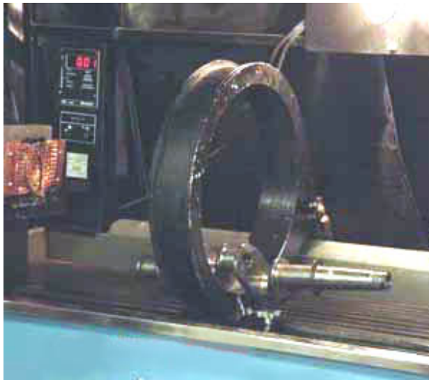
Coil on Wet Horizontal Inspection Unit
