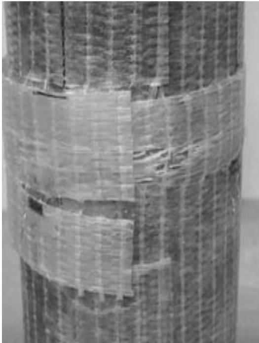
a) Bond delamination between plies
