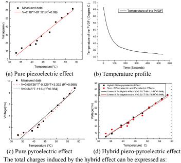
$Q = Q_T + Q_M$ where Q,  $Q_T$  and  $Q_M$  is the total charges induced by the hybrid effect, the pure pyroelectric effect and the pure piezoelectric effect, respectively.
