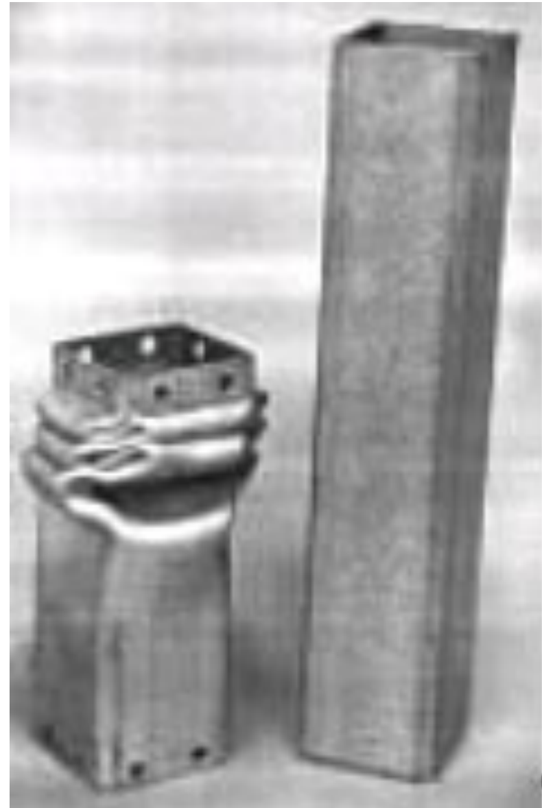
Buckling of a hollow metallic tube
