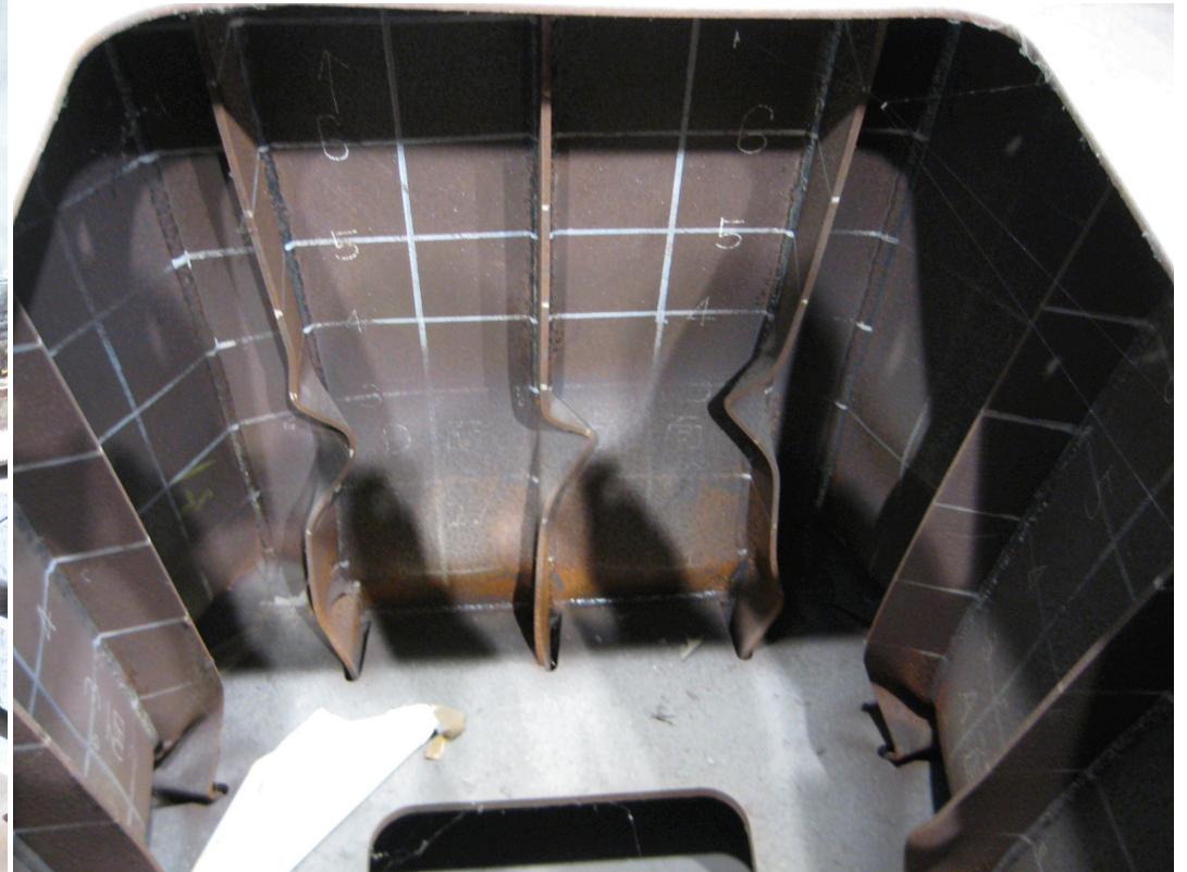
Buckling of a steel column, Public Works Research Institute (PWRI), Tsukuba, Japan (Source: T. Yu)
