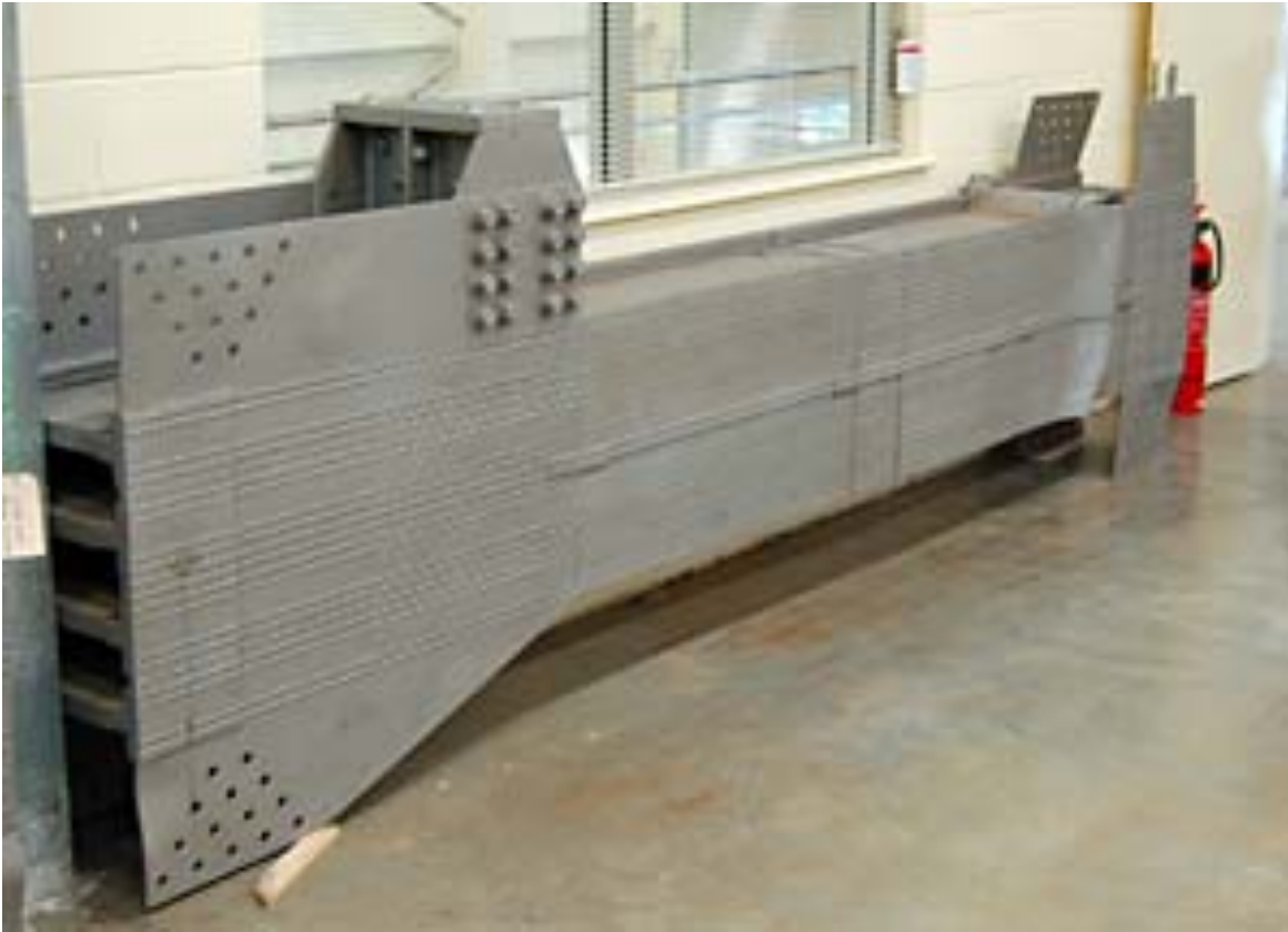
Buckling of a box girder (Source: Unknown)
