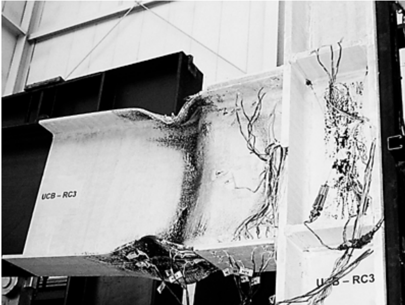
Buckling of an I-beam member (Source: UC Berkeley)
