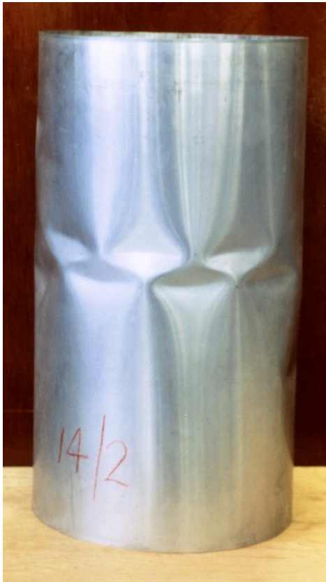
Buckling of an aluminum tube (Source: University of Bath, UK)
