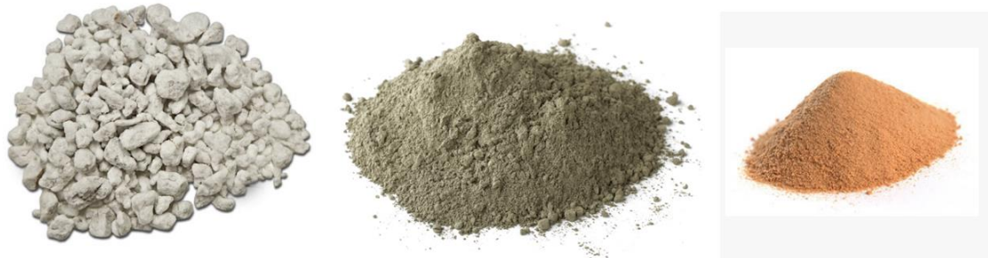
(a) (b) (c) Figure 1. (a) course aggregate (perlite) 1 , (b) cement 2 , (c) fine aggregate 3
