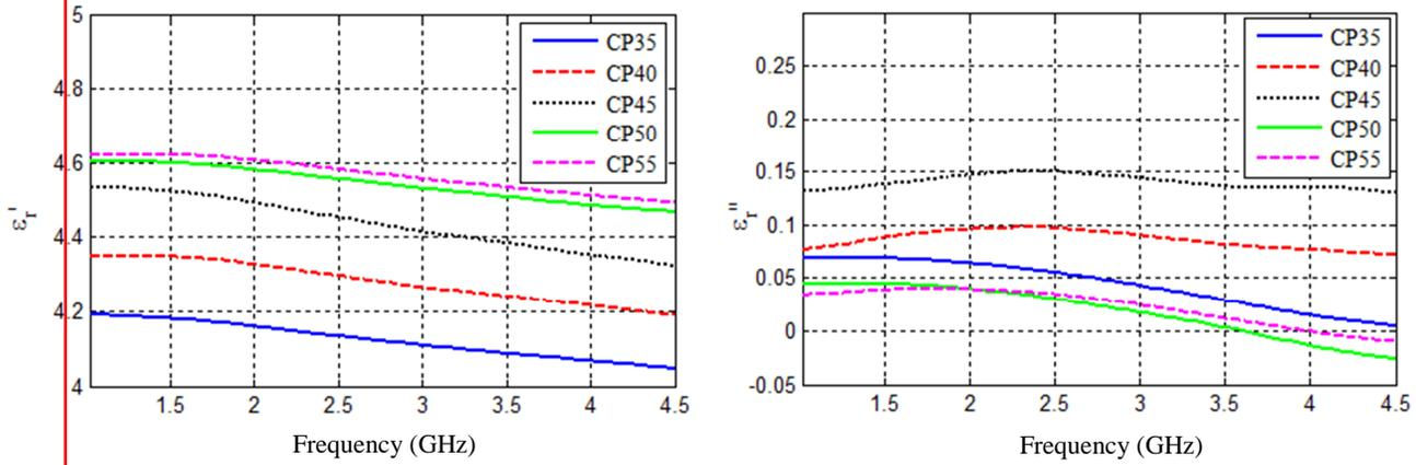
Figure 3: Dielectric measurements of oven-dried cement paste specimens
