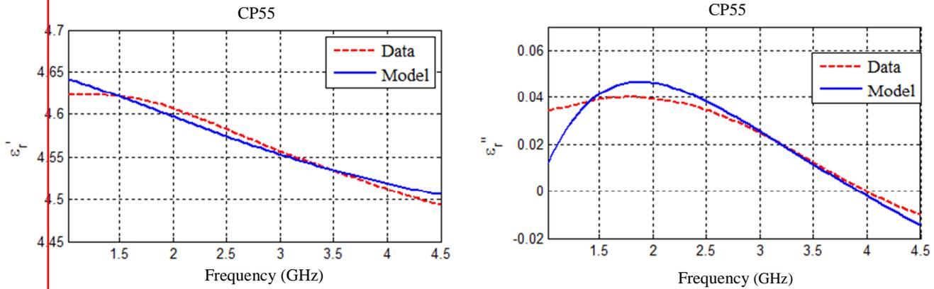
Figure 8: Comparison between the data of the dielectric constant and loss factor and the values obtained by modeling for CP55
