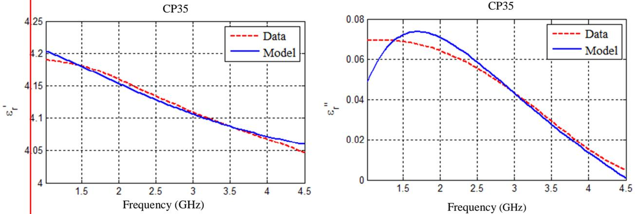
Figure 4: Comparison between the data of the dielectric constant and loss factor and the values obtained by modeling for CP35
