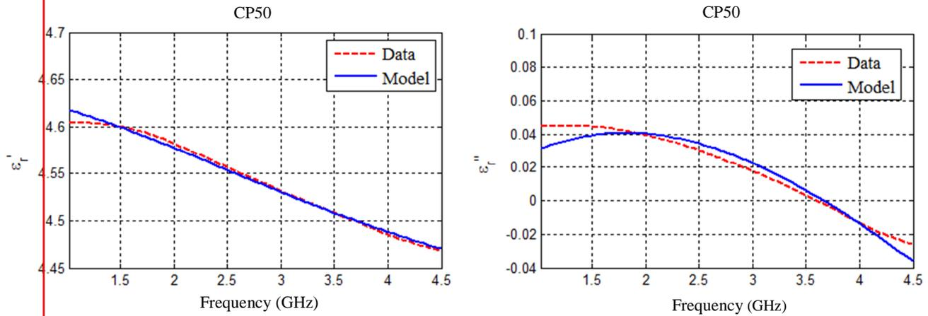
Figure 7: Comparison between the data of the dielectric constant and loss factor and the values obtained by modeling for CP50
