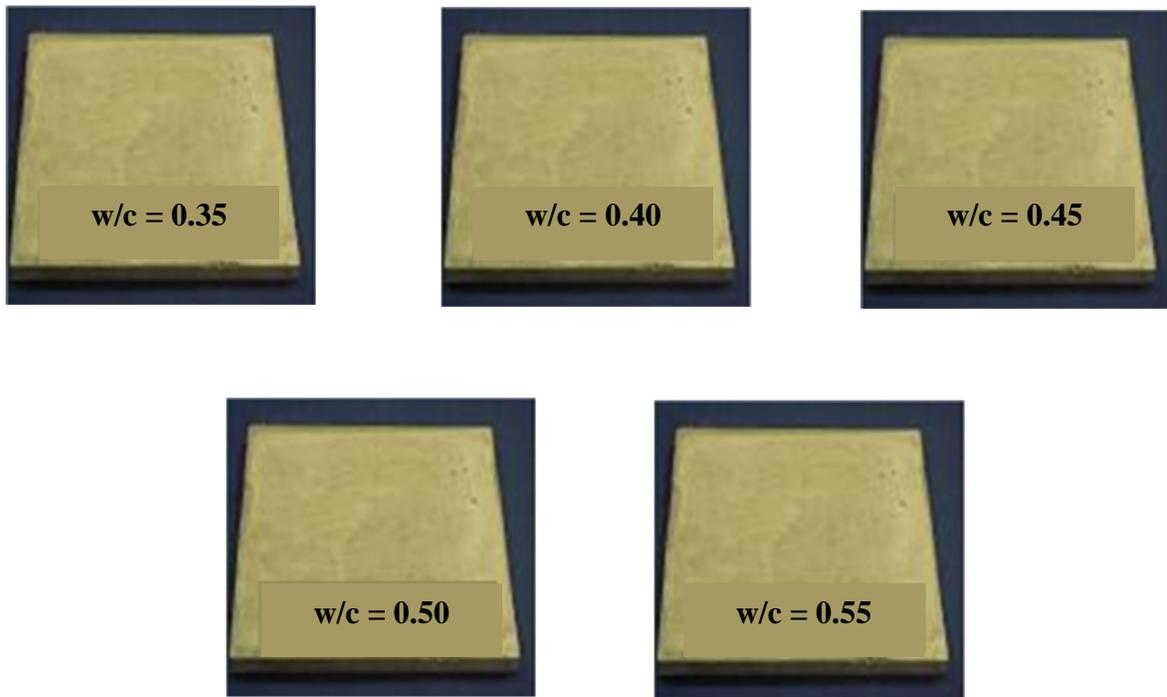
Figure 1: Oven-dried cement paste specimen panels
