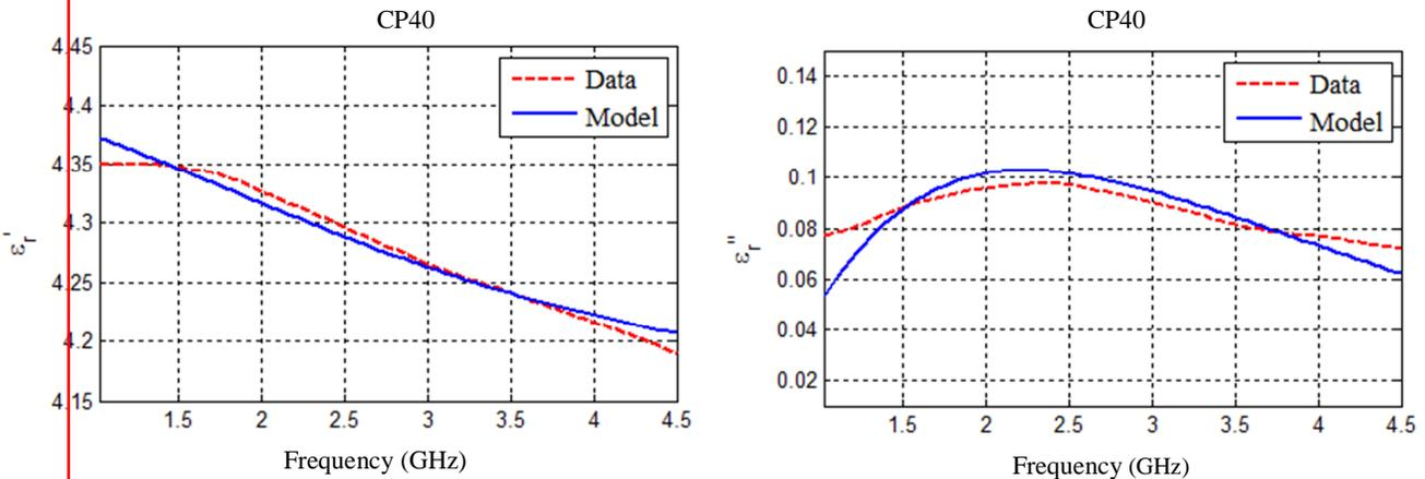
Figure 5: Comparison between the data of the dielectric constant and loss factor and the values obtained by modeling for CP40
