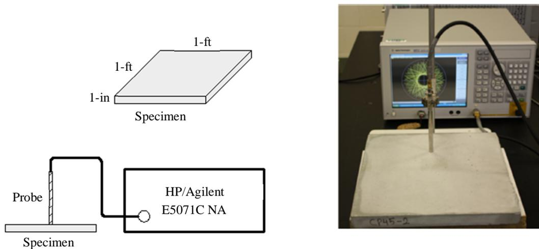
Figure 2: Setup of contact dielectric measurement system and dimensions of specimen
