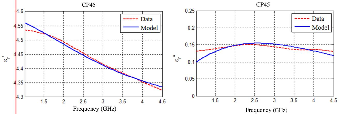
Figure 6: Comparison between the data of the dielectric constant and loss factor and the values obtained by modeling for CP45
