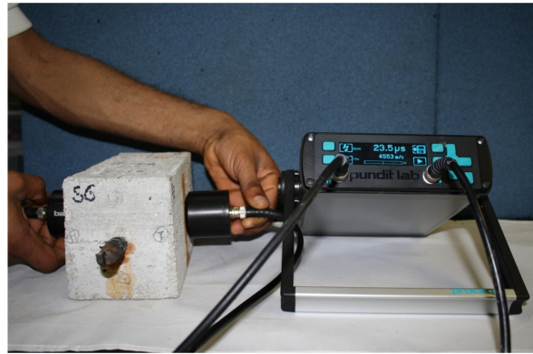
(a) Direct transmission measurement spots (Plan view) (b) Picture of UPV test on corroded reinforced cement mortar
