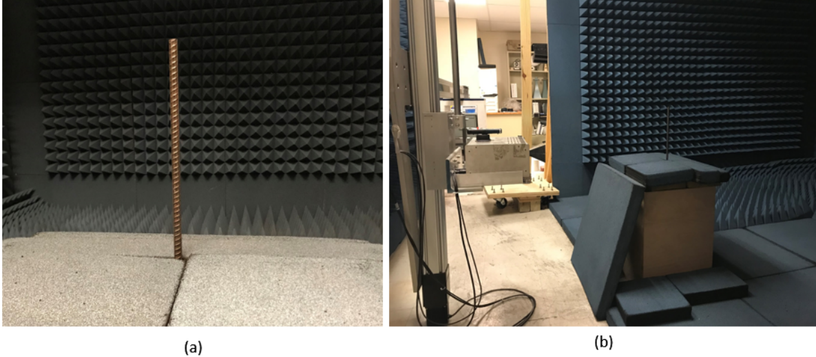
Figure 5: Single steel rebar setup: (a) single rebar located in front of radar, (b) the experiment setup
