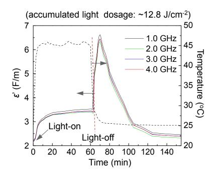
**Figure 6.** Time-dependent relative dielectric constant ( $\varepsilon_r'$ ) profiles of trilayered sample **3–1** at the frequency range of 1.0–4.0 GHz under illumination using a LED white light, showing large photoswitchable amplification of  $\varepsilon_r'$  at the light-off state.
