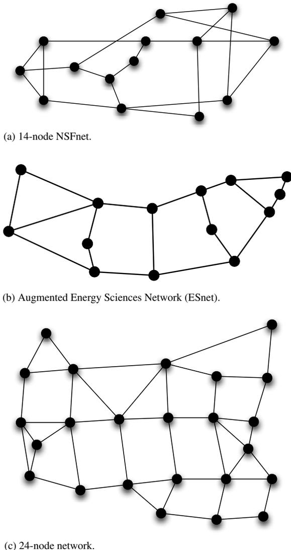
Fig. 3. WDM mesh networks used for heuristic evaluation.
