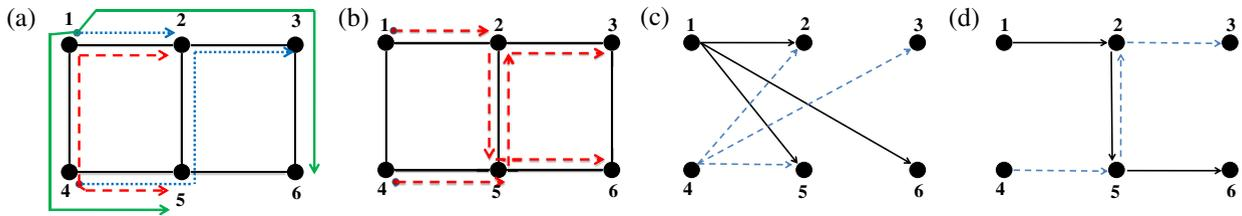
Fig. 1. (Color online) Illustration: number of wavelengths required to satisfy the multicast requests  $R_1 : \{1, (2, 5, 6)\}$  and  $R_2 : \{4, (2, 3, 5)\}$  using (a) MVWU and (b) DMN; the corresponding logical overlays for (c) MVWU and (d) DMN.
