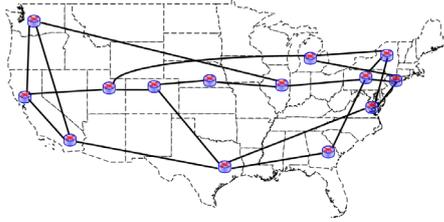
Fig. 2: NSF topology with bidirectional links between the nodes, each carrying  $10 \times 10$ -Gb/s packets.
