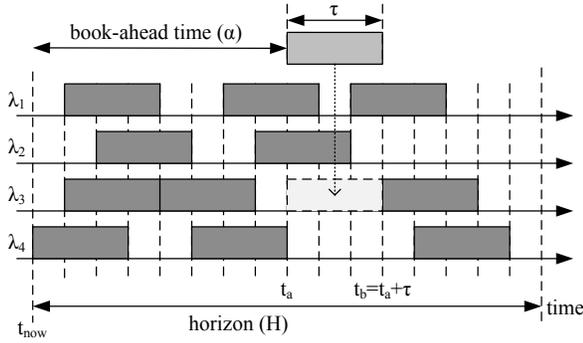
Fig. 3. First-fit slot and wavelength assignment (FF-SWA) policy.
