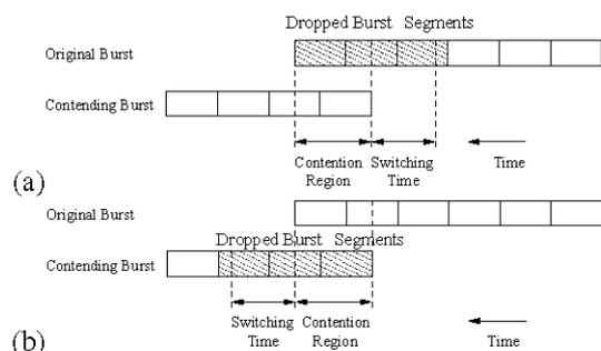
Fig. 1. Selective segment dropping for two contending bursts (a) tail-dropping policy (b) head-dropping policy.
