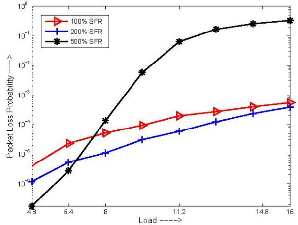
Fig. 6. Packet loss probability vs. network load with very-high serial forward redundancy.
