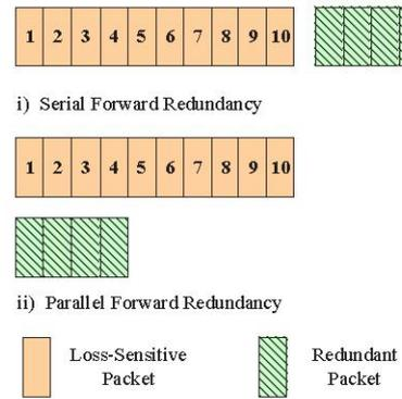
Fig. 2. Different forward redundancy schemes i) serial forward redundancy and ii) parallel forward redundancy.
