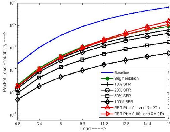
Fig. 4. Packet loss probability vs. network load.
