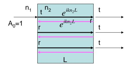
For a resonant filter, n2 = 1.5, n1 = 1,  $L = 20\mu m$ . a). Calculate three of the passing wavelengths around 1.5 $\mu$ m. b). What's the orders (m) of these passing wavelengths? c). What's the wavelength separation?
