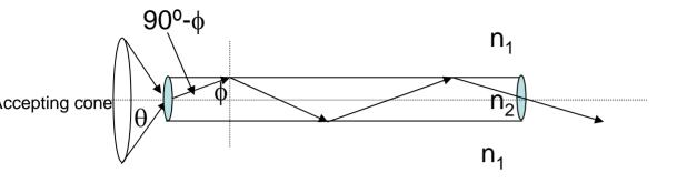
If the index of an optical fiber is  $n_2 = 1.5$  (glass) and  $n_1 = 1.0$  (air). Calculate the maximum allowed angle  $\theta$  for low loss transmission in an optical fiber. Sin( $\theta$ ) is called numerical aperture.
