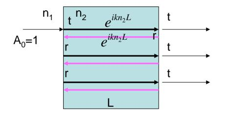
For a resonant filter, n2 = 1.5, n1 = 1, If we want the filter to pass the wavelength of around  $1.5\mu m$ ? what are the possible lengths for the resonator? What's the free spectral range for each of these lengths?
