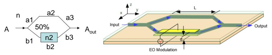
Electro-optic effect,  $n_2$  changes with E –field,  $n_2 = n - 1.5 \times 10^{-4}$ V, and the length L = 2cm. Assume the wavelength of the input light is 1.5µm.
