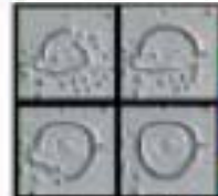
Quantum corral of 48 iron atoms on copper surface positioned one at a time with an STM tip Corral diameter 14 nm
