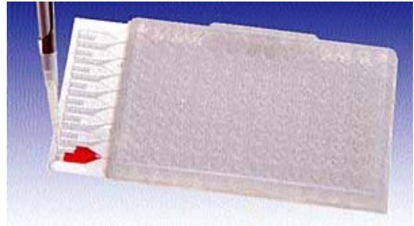
Quantitative gene expression results using a polymerase chain reaction can be obtained with this microfluidic card by pipetting in reaction mixes, centrifuging, sealing, removing the reservoir, and thermal cycling.
